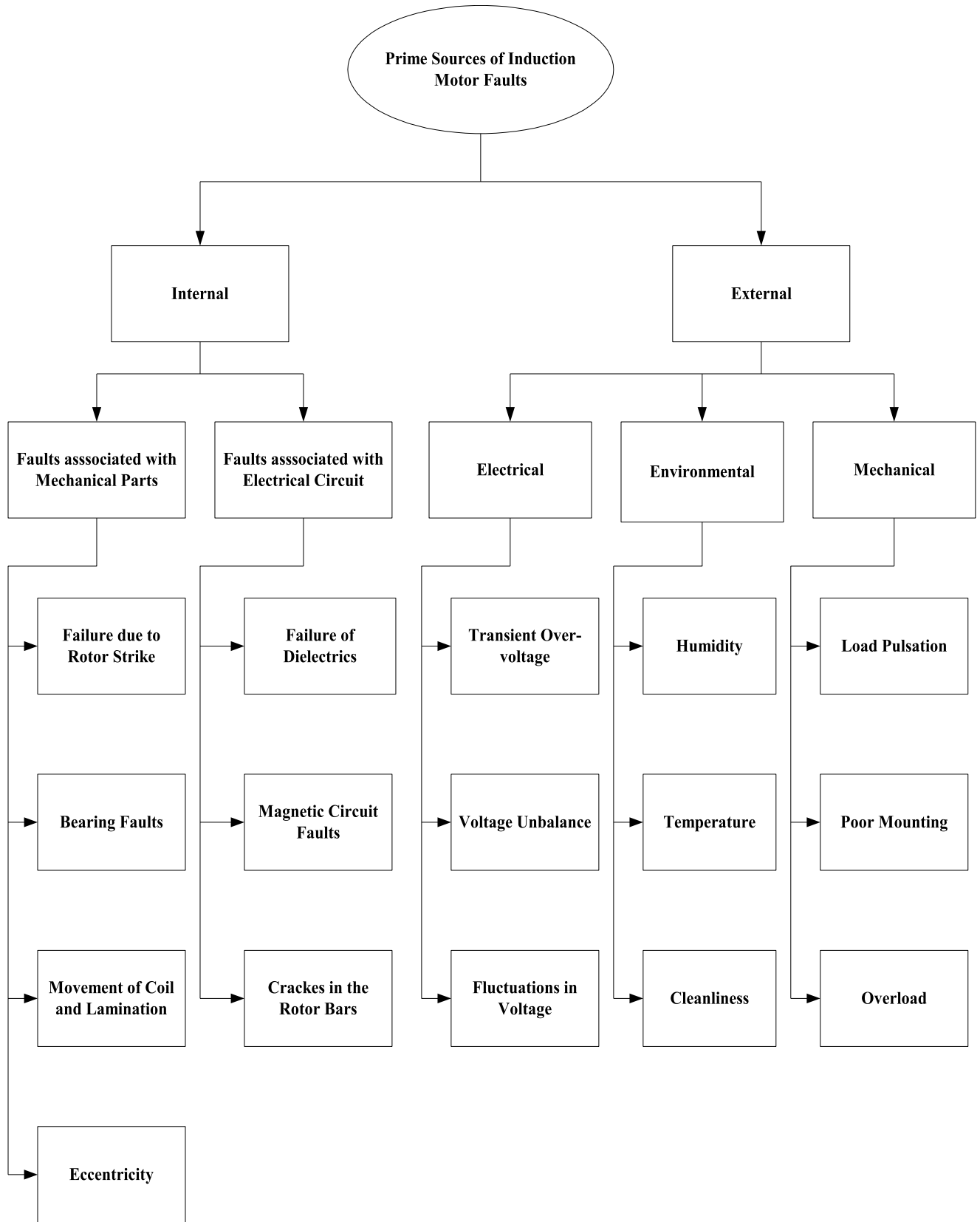
FIGURE 4. Prime sources of induction motor faults.
