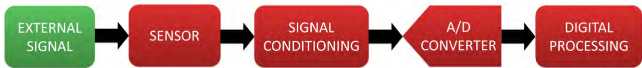
FIGURE 1. Block diagram of a typical digital system processing real-world signals.
