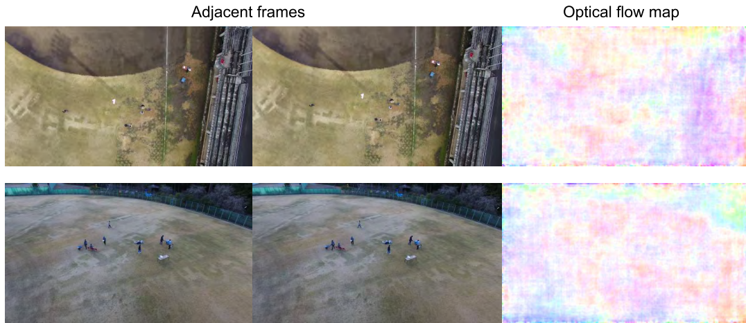
FIGURE 5. Visualizations of optical flow maps generated by PWC-Net [26], using Okutama-action Dataset. Due to the tiny size of person and the drone camera movement, it is challenging to obtain person motion information from the optical flow.
