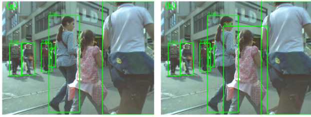
FIGURE 3. Detection results with NMS (a) and Soft-NMS (b).
