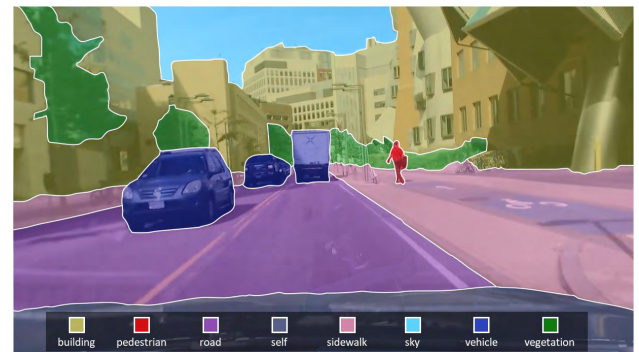
(c) Forward-Facing Camera for Driving Scene Perception.
