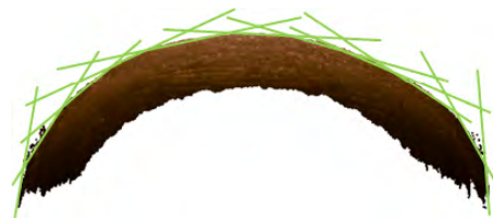
FIGURE 5. Shows the pressure simulation lines. Pressure will be simulated along the normal of each line. Increasing the number of slices will produce a genuine rolling effect but, increases computational cost.
