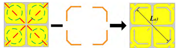
FIGURE 4. Configuration of the BEDPA. (unit: mm, L_{a3} = 71.5 ).
