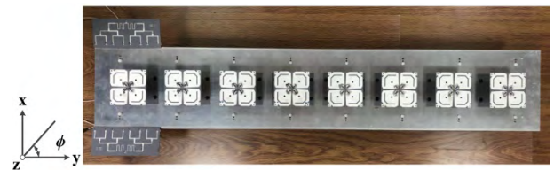
FIGURE 15. Prototype of linear array with the BEDPA.
