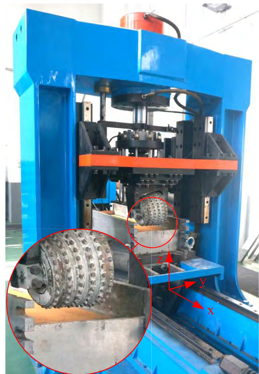
FIGURE 27. Experimental equipment for rock breaking with tipped hob cutter.
