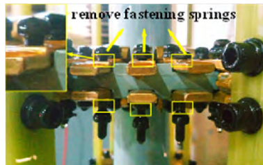
d. Simulating the loosening of transition contact
