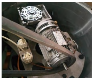
FIGURE 5. Simulating a motor jam fault in SYJZZ-35 OLTC.
