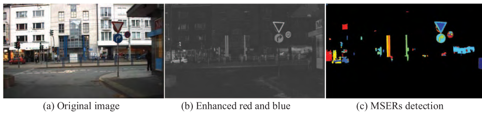
FIGURE 4. Re-implemented MSERs_NRB detection method in [48]. (a) is the original input image. (b) red and blue enhanced image of MSERs_NRB. (c) detection result of MSERs_NRB. The results were gotten with a threshold of 1.5.
