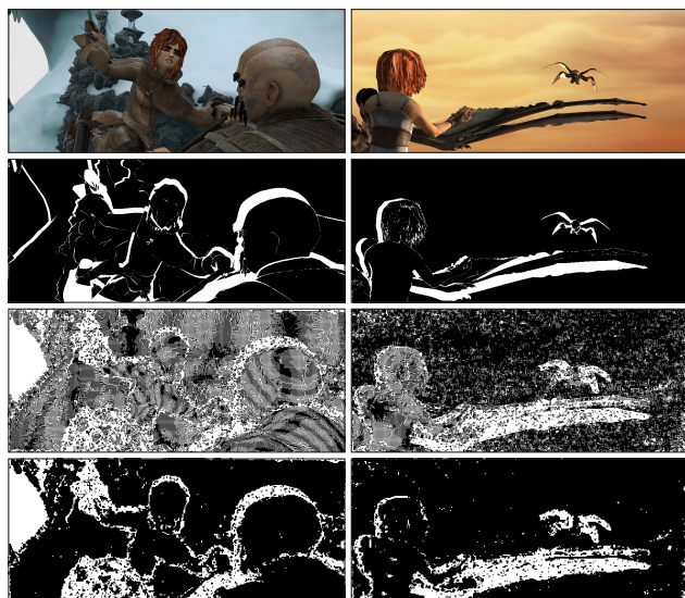
FIGURE 4. Comparison of results of occlusion detection. From left to right: The sequences of ambush_6 and temple_3 from the MPI-Sintel dataset; from top to bottom: The mean of two consecutive images, ground truth of occlusions, results of article [40] and results of the proposed method.
