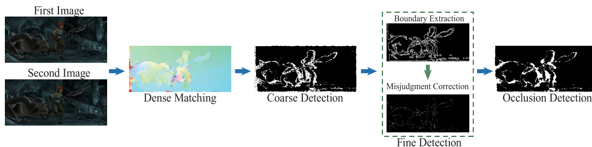
FIGURE 2. Overview of the proposed TSOD algorithm. Given two images, we compute dense matches using CPM [14]. We use the statistical dense matching method to detect most false matches (Coarse Detection) and correct misjudgment matches using a descriptor-based triangulation (Fine Detection).
