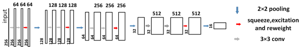
FIGURE 5. In the encoder, U-Net and SE-Net are combined by adding SE-Net modules in front of each pool layer.
