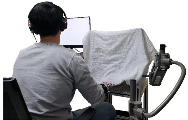
FIGURE 2. The experimental setup. A participant wears headphones where white noise is played. S/he inserted thumb and index finger in the experimental apparatus and the arm is placed on an armrest to minimize the fatigue. During the experiment, white cloth covered the hand to block any possible visual cue from the haptic interface.
