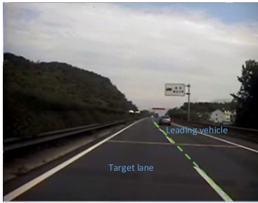
FIGURE 5. The initial moment of the lane change behavior of the leading vehicle.
