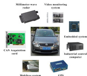
FIGURE 3. Components of the test platform.
