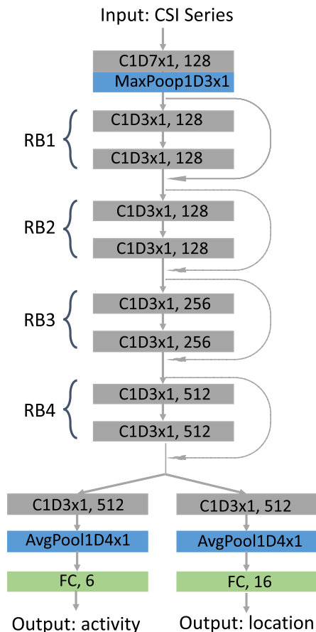
FIGURE 11. Deep framework. ‘RB’ is the abbreviation of residual block. For all RBs having one residual shortcut, we term this framework as ResNet1D-[1,1,1,1].
