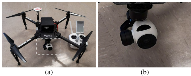
FIGURE 6. Unmanned aerial vehicle used for data acquisition: (a) DJI Matrice 100 and (b) DJI Zenmuse X3 multispectral sensor (B-G-NIR).
