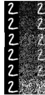
FIGURE 2. Adversarial examples produced by FGSM with different \epsilon (0.1 – 0.6), and \epsilon increased 0.1 by line. In each line, the left side is the normal examples, the middle is the designed noise, and the right side is the adversarial examples.
