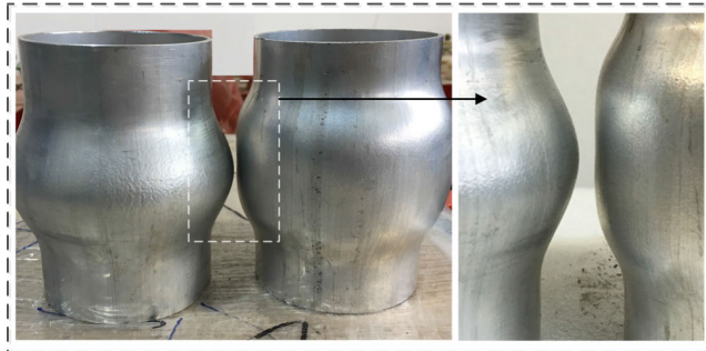
FIGURE 13. Photos of the Expanded tube after discharging with a system of helix coil and concave coil.
