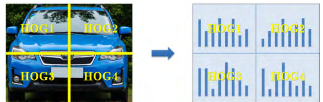
FIGURE 5. symmetry of HOG feature in an image.
