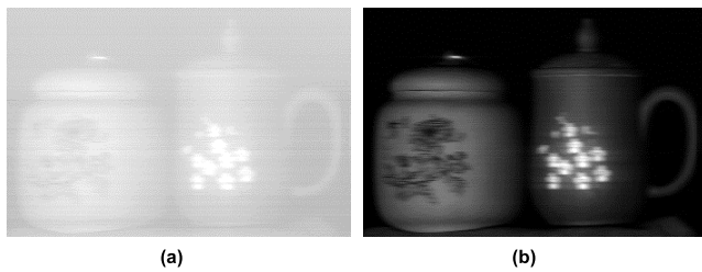
FIGURE 3. The integration images of (a) result before elimination of the back scattered light and (b) result after elimination of the back scattered light.
