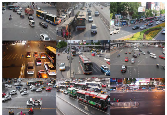
FIGURE 1. Sample images of the UA-DETRAC benchmark data-set [9] that contain various challenges on vehicle detection such as weather conditions, varying times, large scale changes and occlusions.
