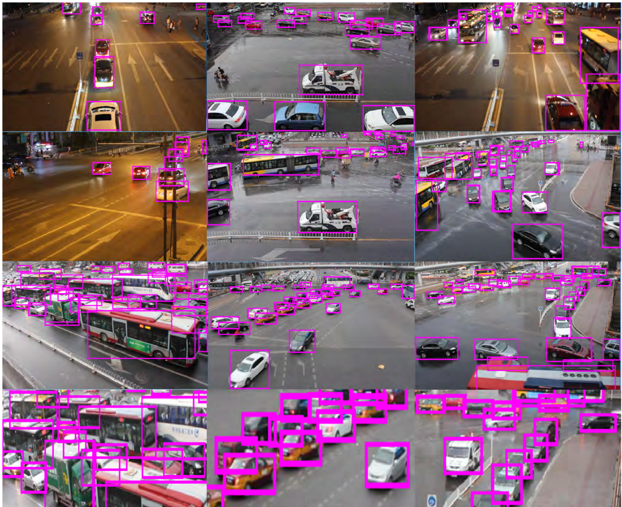
FIGURE 6. Qualitative detection results of out proposed method on the UA-DETRAC benchmark test-set. The result bounding boxes are dense around heavy occluded vehicles and correctly detected for hard traffic scene.
