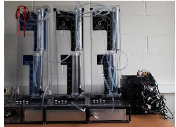
FIGURE 21. Photo of the sextuple water tank system.
