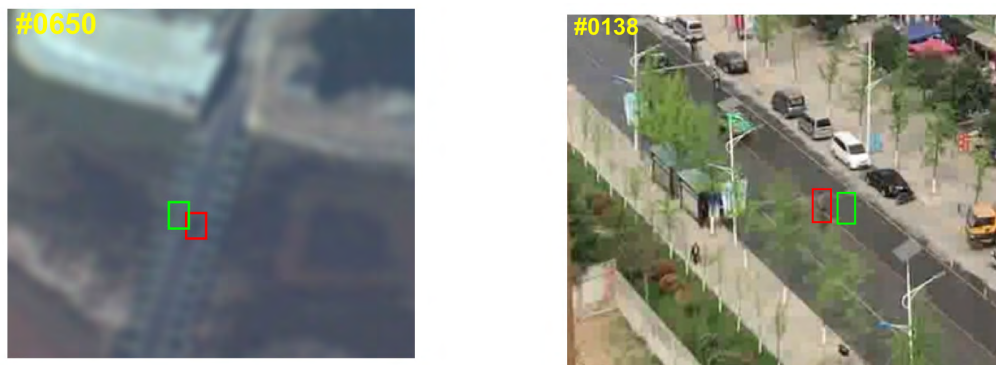
FIGURE 8. Failure cases for the proposed method. Red and green bounding boxes denote the ground-truth and our result, respectively.
