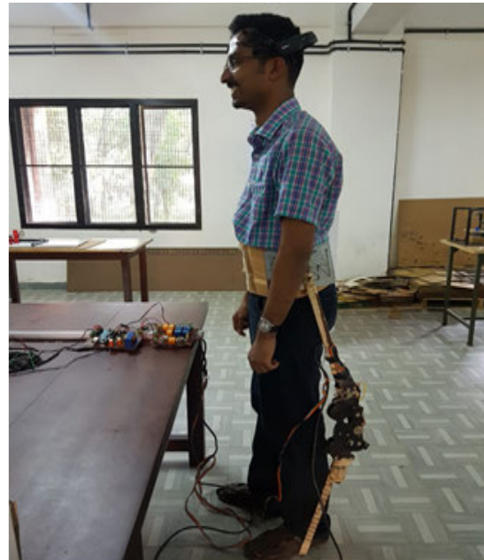
FIGURE 9. Controlling the outer structure of exoskeleton using EEG headset.
