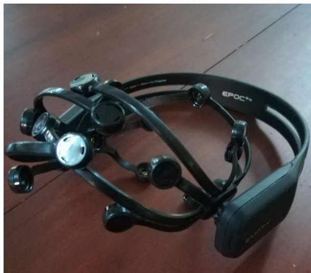
FIGURE 2. Emotive EPOC mobile EEG headset.
