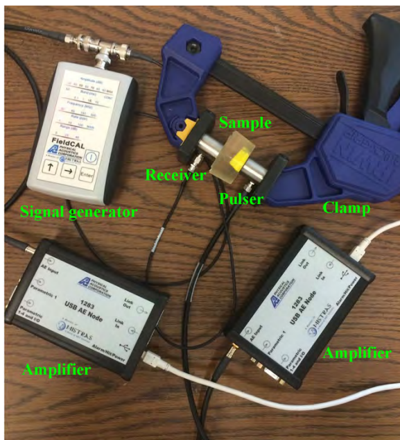
FIGURE 9. Sound test on the sample. One transducer serves as the pulser and the other serves as the receiver. The incidence of a 30 kHz sine tone burst is generated by the signal generator.
