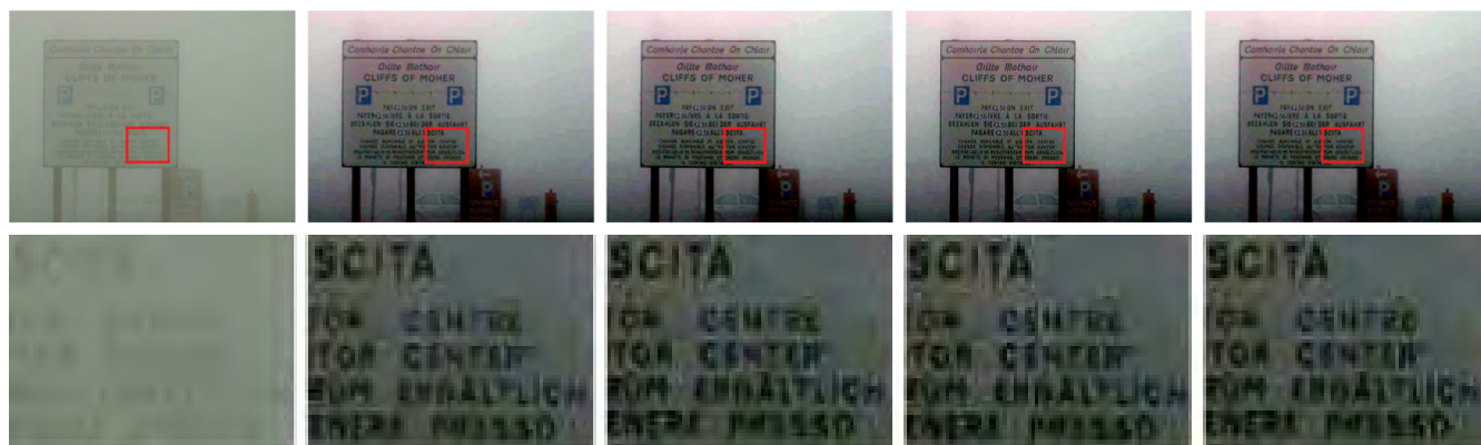
FIGURE 3. The first row is the original image, and the defogged images of MSRCR when the number of kernels is 3, 6, 9 and 12, respectively. The second row is the local amplification effect of the red box area in the first column.
