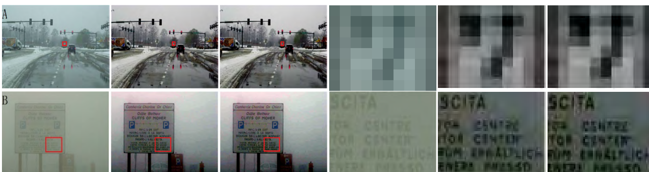
FIGURE 4. From left to right: the original images A and B, and the defogged images are obtained by MSRCR, multi-channel convolution, the local amplification effect of the red box of the original images, the local amplification effect of the red box of the defogged images are obtained by MSRCR, and multi-channel convolution.
