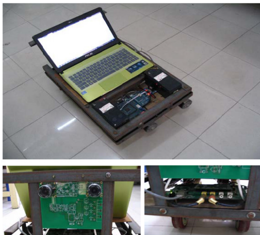
FIGURE 1. (Top) Our mobile robot platform. (Bottom row) Binocular visual system and DM642 image processing card.
