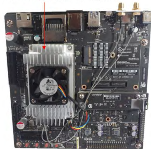
FIGURE 19. Jetson TX2 embedded system.
