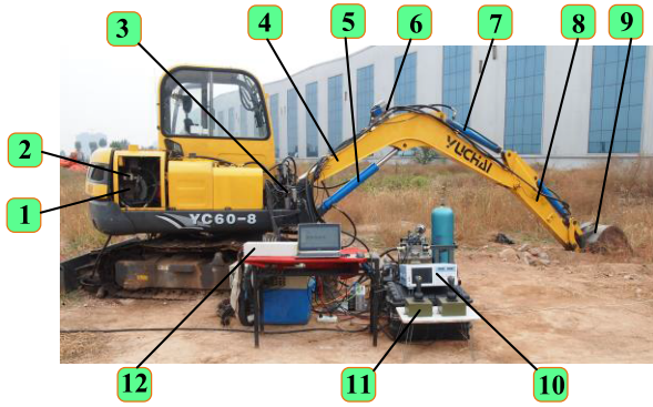
FIGURE 11. Test prototype and system components. 1-Pressure and flow control pump; 2-Electric motor; 3- Boom control valves; 4-Boom; 5-Boom cylinder; 6- Arm control valves; 7-Arm cylinder; 8-Arm; 9-Bucket; 10-Power meter; 11-Joysticks; 12-dSPACE.
