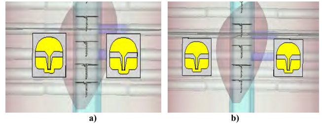
FIGURE 12. Location of the antennas respect to the sternotomy wires as the antennas separation distance is (a) 10 cm and (b) 15 cm in the case of the symmetric antenna location option.
