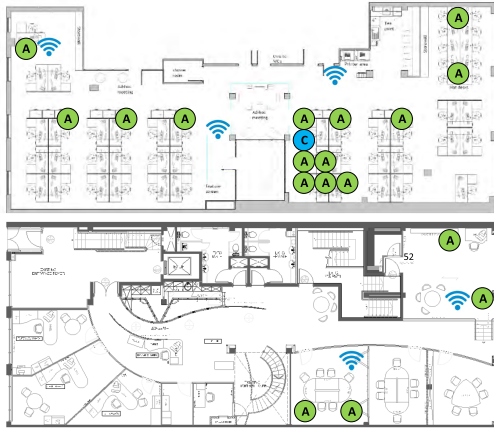
FIGURE 15. 19 Node TelosB Testbed. Initiating nodes are marked in green, and the SDN controller in blue.
