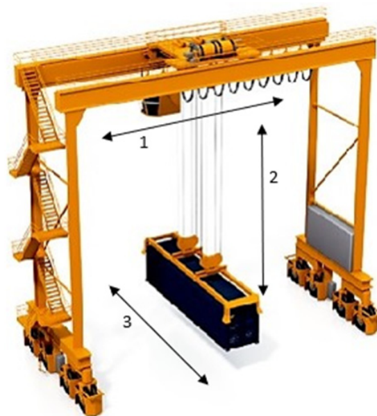
FIGURE 1. Directions of motions of RTG crane (1-Trolley, 2-Hoist, 3-Gantry).
