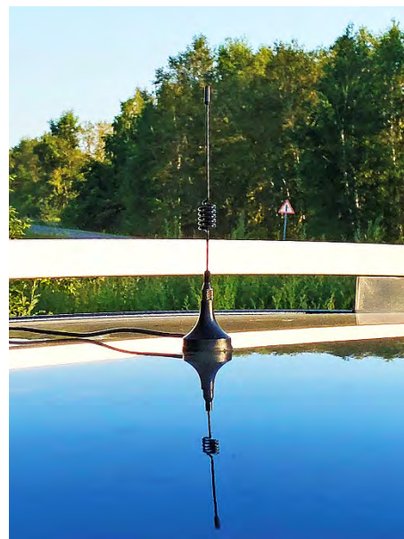
FIGURE 7. The 434 MHz antenna mounted on the roof of the car during the outdoor experiments.
