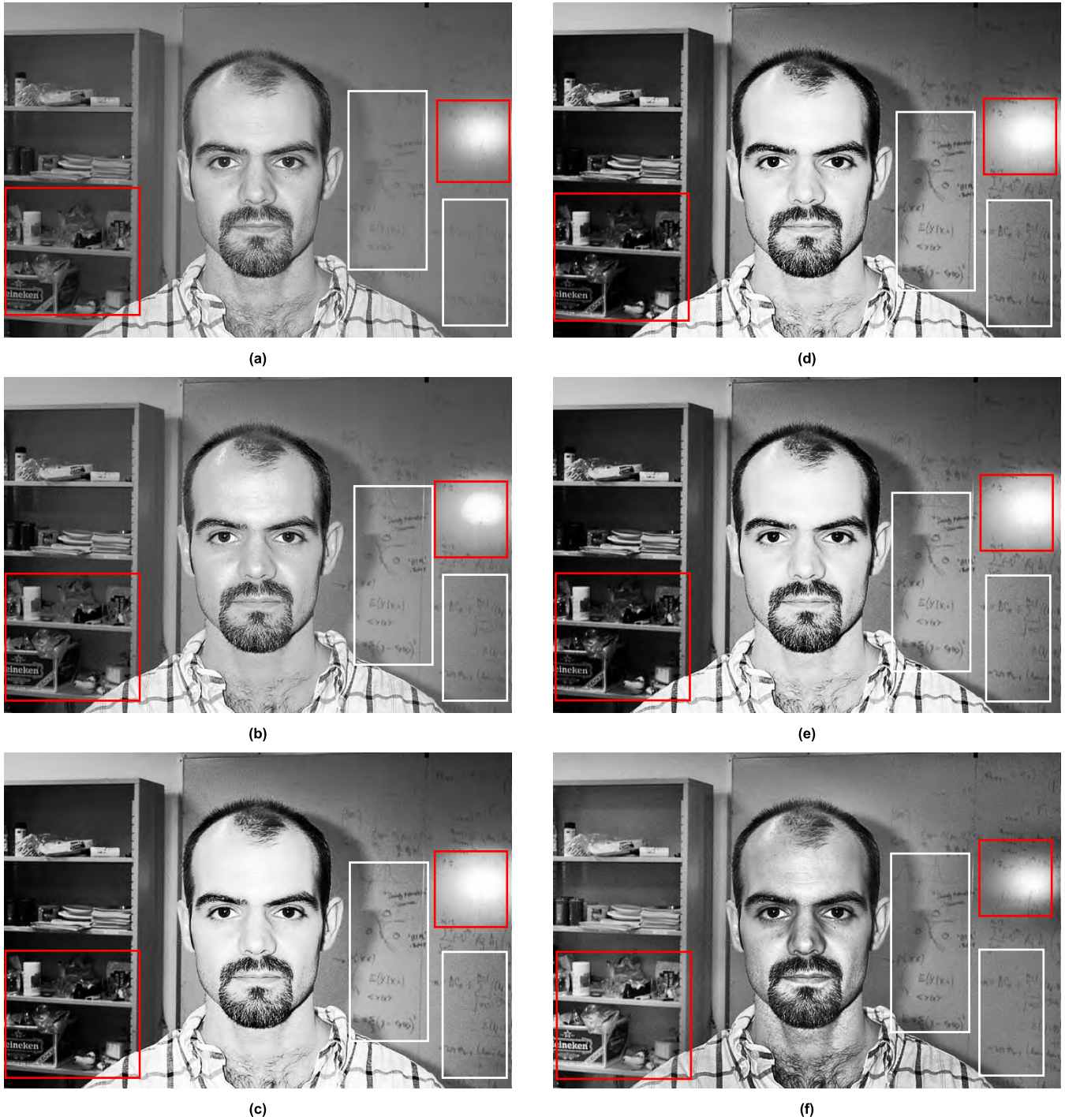
FIGURE 18. (a) Original image of CloseupSample2 and resultant images produced by (b) ERMHE, (c) GHE, (d) BBHE, (e) DSIHE and (f) CLAHE with metric scores (PSNR, ICF, DE and AMBE) computed for each image.
