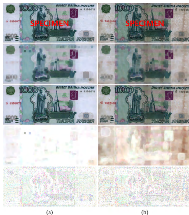
FIGURE 2. Soiling pattern extraction examples of (a) fit banknote and (b) unfit banknote. From the first to fifth row: Original, morphologically closed, modified dynamic closed, large-scale soiling pattern, small-scale soiling pattern images.
