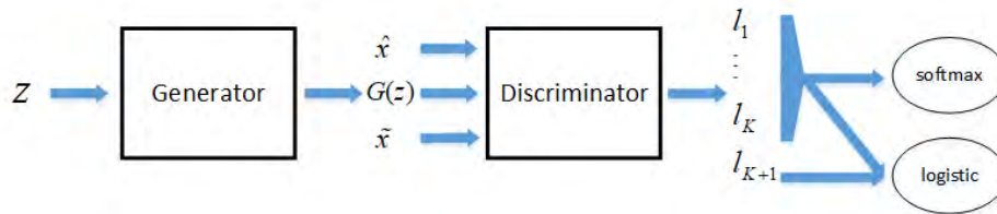
FIGURE 1. Semi-supervised learning based on GAN. The discriminator D outputs a K + 1 dimensional vector L . The first K elements represent the score of the input belonging to each category. The last one represent the score of the input belonging to G(z) .
