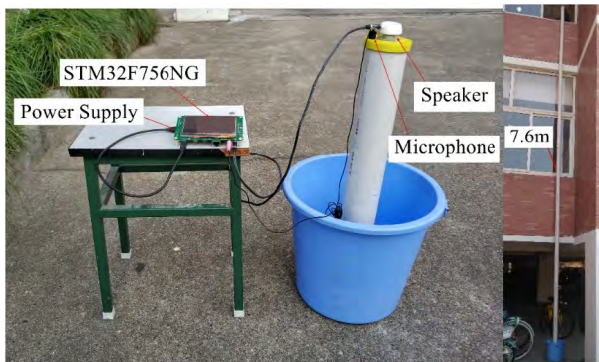
FIGURE 13. Hardware set-up of the level gauge.
