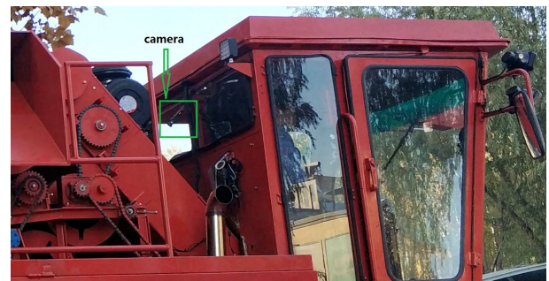
FIGURE 1. A real-time monitoring system in a corn harvesting machine. The camera is mounted on a fixed bracket above the conveyor belt to collect images.
