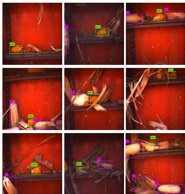
FIGURE 10. Some detection result on the test set. We show some detection examples with classification scores higher than 0.5. The green and purple bounding boxes represent broken and non-broken corns, respectively.
