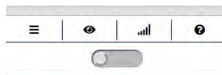
FIGURE 3. Latent web browser extension acquisition control UI. On top, from left to right, the buttons are: Open options page; turn on/off the acquisition preview; open the acquisition results page; “about” information. The bottom button is to start/stop the acquisitions.
