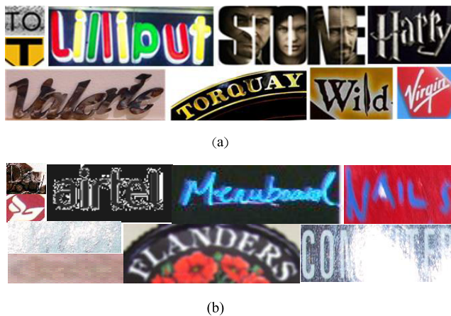
FIGURE 6. (a) Correct and (b) incorrect samples recognized under the CTC-Attention joint mechanism.
