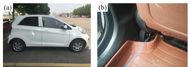
FIGURE 8. Onsite test of vehicle dynamics. (a) Test vehicle; (b) Sensor arrangement of the car body vertical acceleration.
