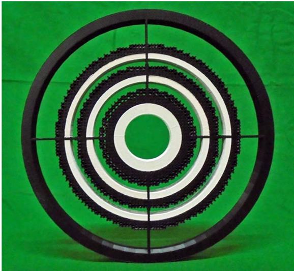
FIGURE 9. PREMIX and ABS 1X FDM lens (radius = 90mm).
