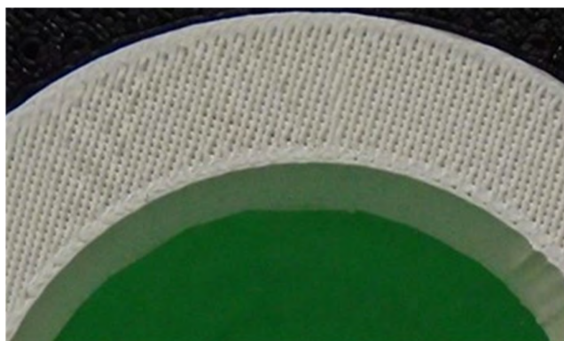
FIGURE 5. Linear infill pattern used to vary infill percentage.
