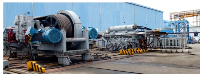
FIGURE 3. Winch and integrated cylinder of the semi-active heave compensation system.
