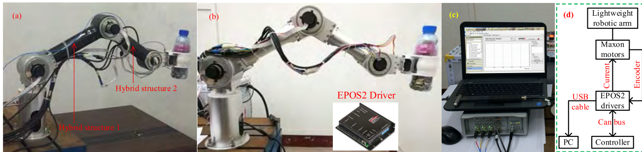
FIGURE 12. (a) Experimental prototype of the lightweight CFRP/AA arm, (b) Experimental prototype of the lightweight AA arm, (c) EPOS-studio in PC, and (d) schematic of torque measurement.
