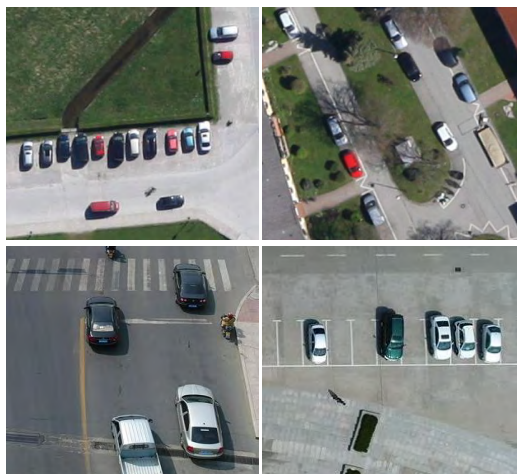
FIGURE 1. Example of some difficulties in vehicle detection (arbitrary orientation, small size of vehicles, and complex background in aerial images).
