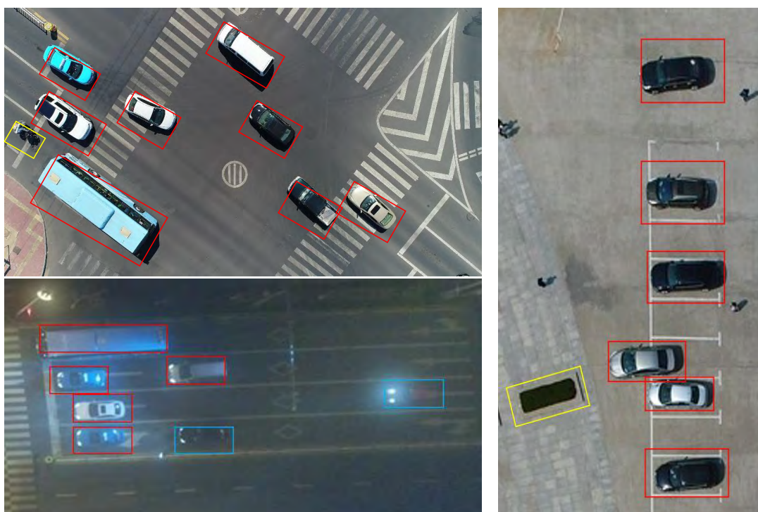
FIGURE 10. Detection and annotation results from the UAVDT. A red box denotes correct localization, a yellow box denotes false alarm and a blue box denotes missing detection.
