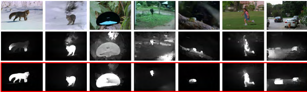
FIGURE 8. Demonstration of performance improvement brought by our novel learning scheme. The middle row demonstrates the low-level saliency results computed by Eq. A5, and the bottom row shows the video saliency performance of our newly-developed learning scheme.
