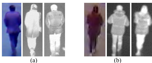
FIGURE 9. Examples of incorrect ReID test result on DBPerson-Recog-DB1: (a) example recorded with rank 3 (left image is probe image, middle image is negative image of gallery set recorded with rank 1, and right image is positive image of gallery set recorded with rank 3) and (b) example recorded with rank 16 (left image is probe image, middle image is negative image of gallery set recorded with rank 1, and right image is positive image of gallery set recorded with rank 16).
