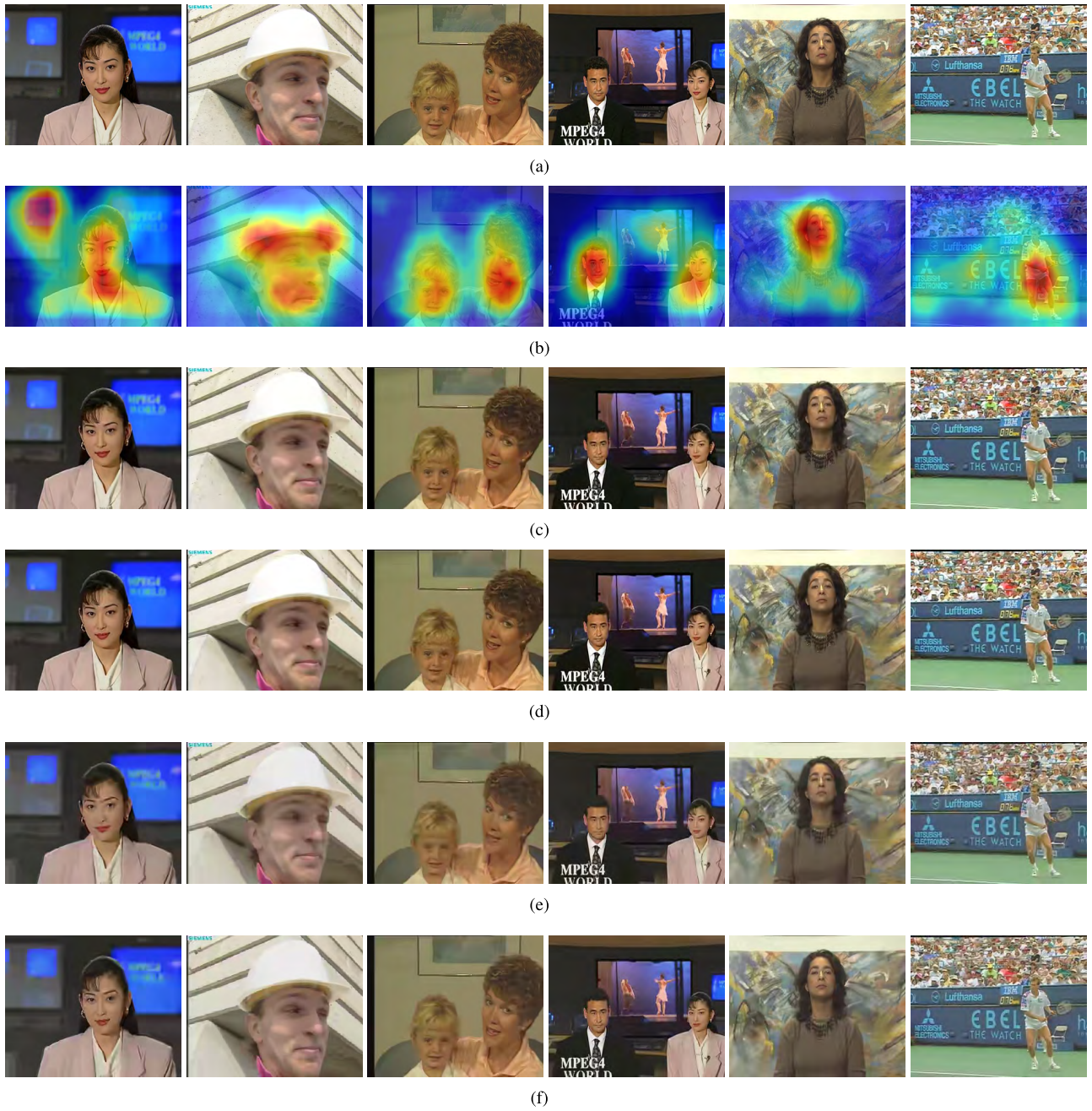
FIGURE 5. Experimental results of the proposed method compared with HEVC for six video sequences: (a) original video sequence (Akiyo, Foreman, Mother-daughter, News, Silent, Stefan), (b) heat map, (c) HEVC coding results with QP = 32, (d) proposed method coding result with QP = 32, m = 6 and n = 0.5 , (e) HEVC coding results with QP = 37 and (f) proposed method coding result with QP = 37, m = 4 and n = 0 .
