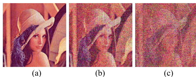
FIGURE 11. Rotation attack results, (a) recovered image of rotation 2°, (b) recovered image of rotation 18°, (c) recovered image of rotation 25°.
